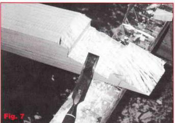
Mark and cut matching shoulder-less tenons on the ends of the frame beam (Fig. 8). Remove enough waste from each side to give a 50 mm wide tenon. The tenons should be about 100 mm long so they will extend 10 mm beyond the frame sides when assembled.
