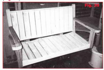
Install two galvanised screw eyes at each end of the swing seat. These are screwed into the top of the rear corners and through the armrest into the front corner.
