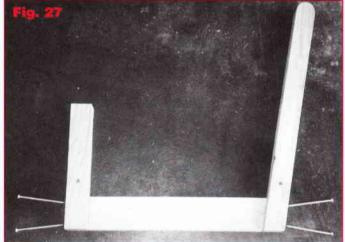
The end rails finish flush with the inside faces of the corners. Use two 100mm treated pine screws at each joint. Glue and assemble parts for both ends of the seat.
