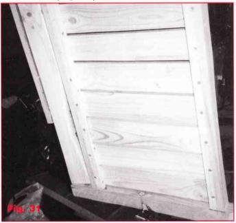
Cut, glue and screw the seat slats (O) in place in the same way using 50 mm screws driven from underneath.
