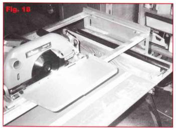
The seat end rails (H) and rear corners (F) have a 10 degree angle cut in their ends. Do this on the workcentre in tablesaw mode with the protractor (Fig. 19).
