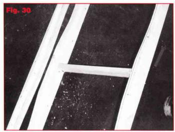
Glue and screw it in place with one 75 mm screw at the front and one at the back, slightly off-centre so they will be hidden under the seat slats. Counterbore the front screw so it can be covered with a wood plug later. The rear screw can be left flush with the rear seat rail.
